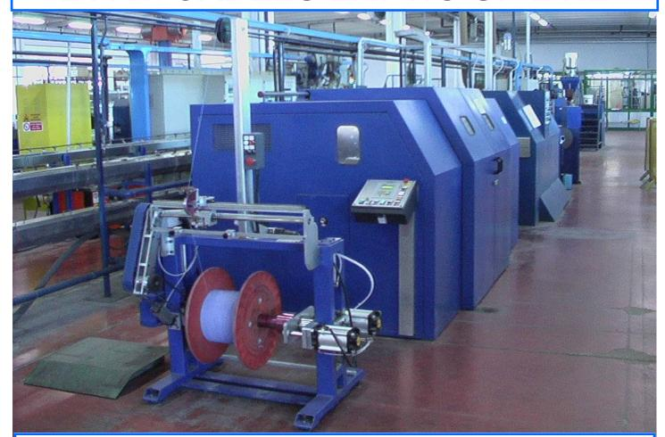
LINE FOR TWINNING AND LAYING-UP L.A.N, U.T.P. AND S.T.P. CABLES
